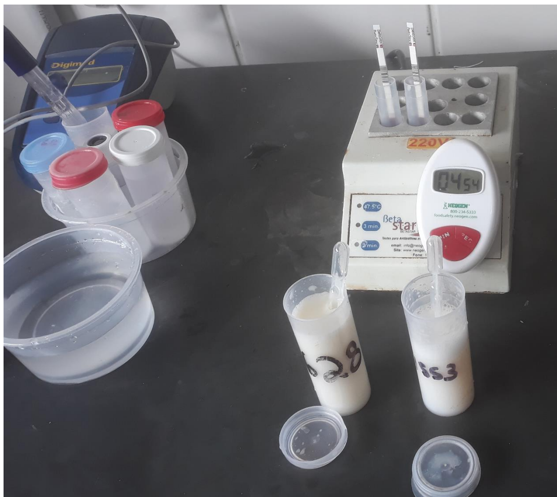
Figure S1: Equipment used in the test to determine the presence of ceftiofur residues.
