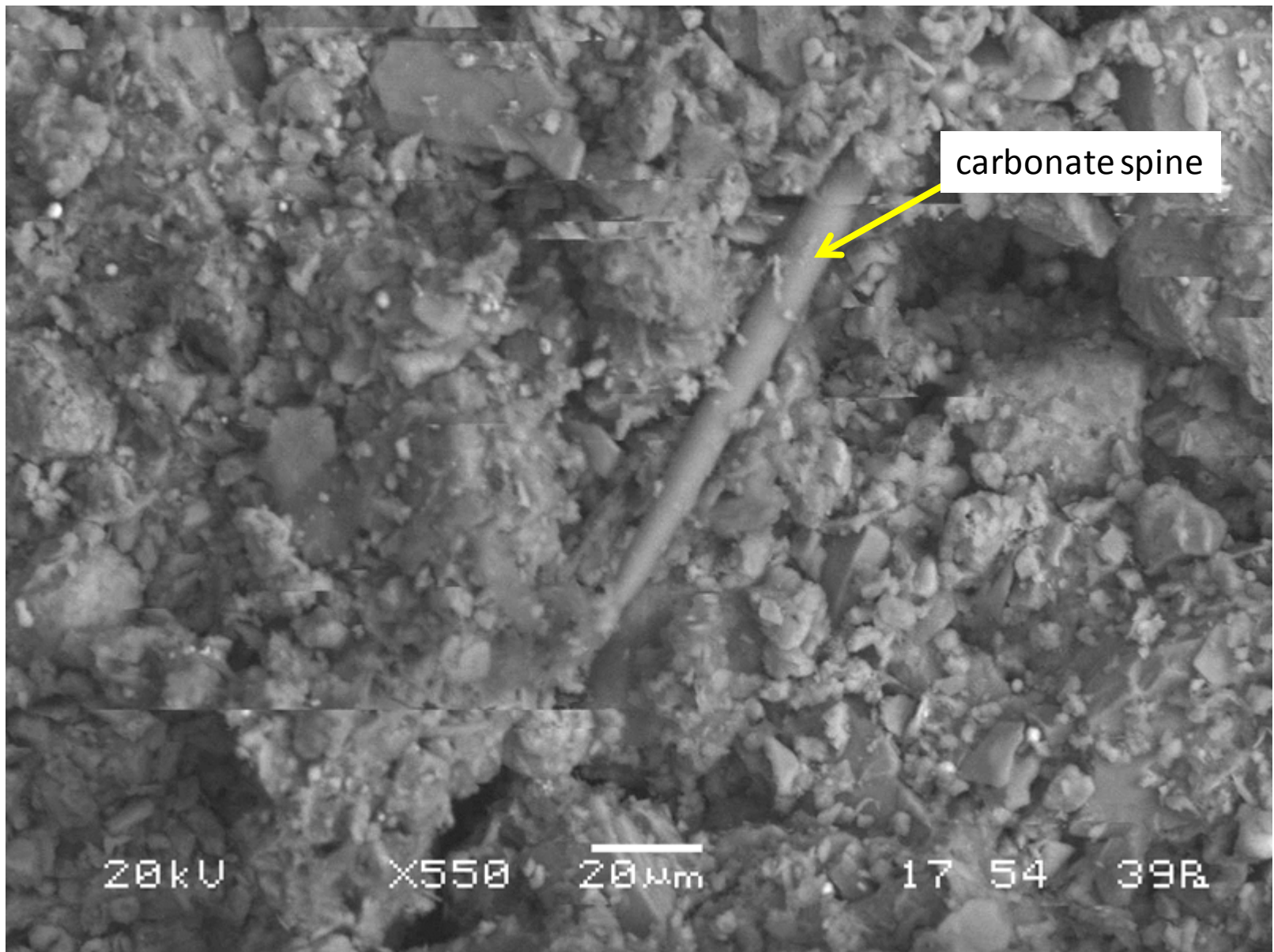
P2 – calcium carbonate spine or spicule; mineral grains include quartz, chlorite, calcite and dolomite; very fine sand, silt and clay sizes
