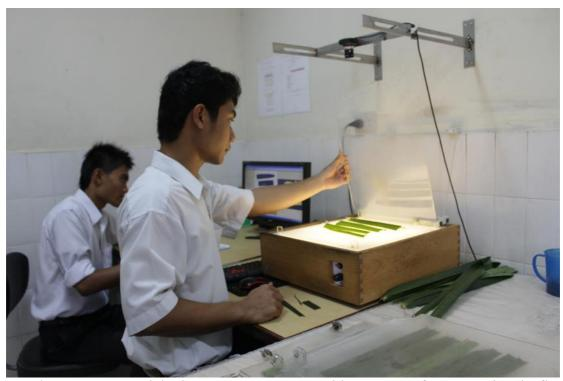
Supplementary Material Figure S1. IDS  $\mu$ Eye video camera for measuring leaflet areas. Note that the freshly-cut pieces of leaflets are constrained by a glass plate before area measurements.
