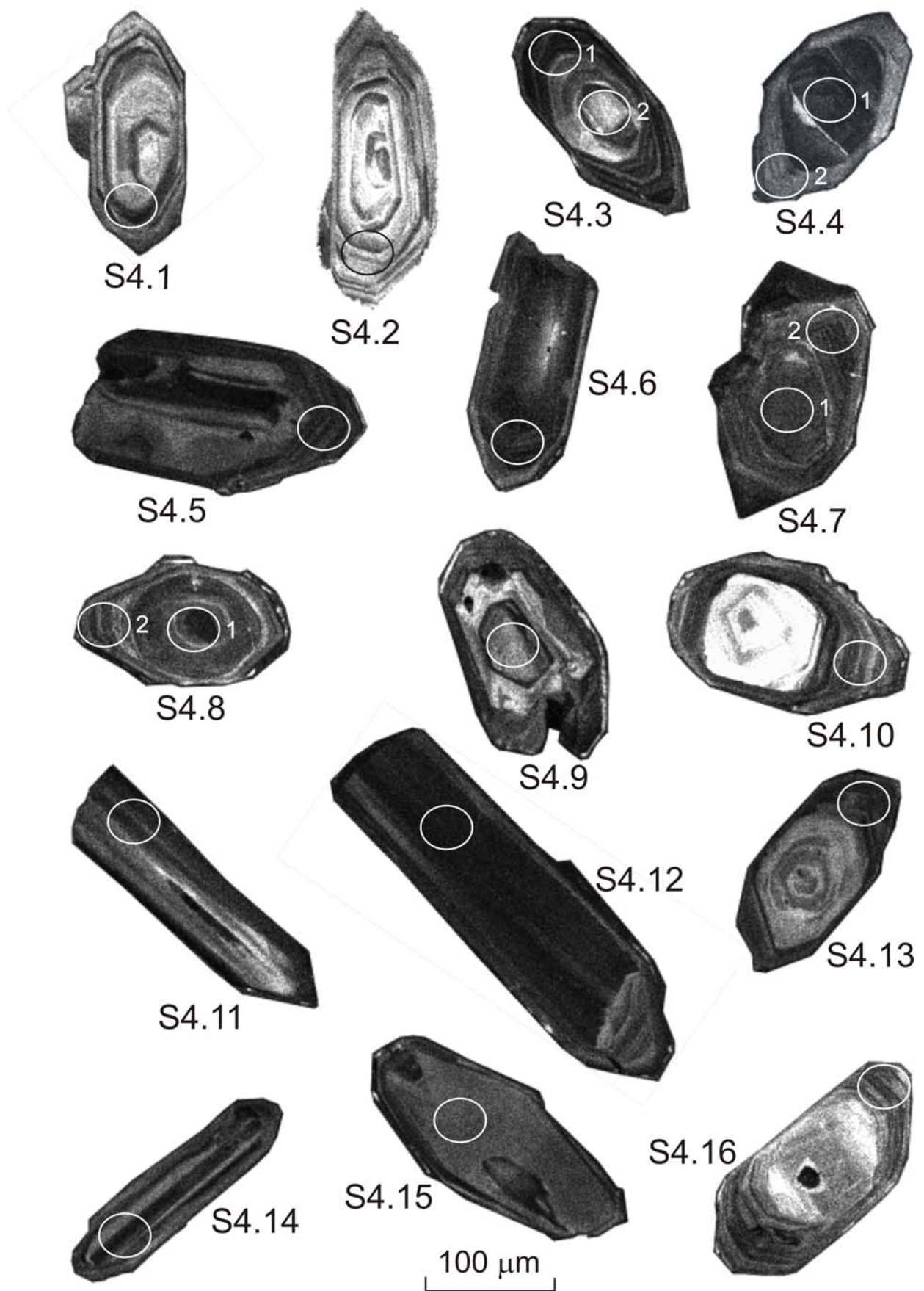
Figure A6. (c) Cathodoluminescence images of zircons with SHRIMP analytical spots from gneiss sample S4.
