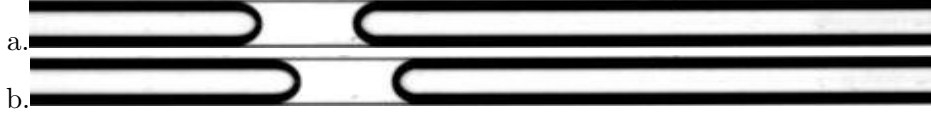
FIG. 1: Movie S1 : Movie showing the temporal evolution of a single liquid plug of initial length L_0 = 1.05mm pushed with the cyclic flow rate forcing in a cylindrical capillary tube of radius R_c = 0.47mm . The movie was shot with a Photron SA3 high speed camera mounted on a Z16 Leica Microscope at a frame rate of 125 images per second, a trigger time of 1/3000s and a resolution of 1024 \times 64 pixels. a. Initial state b. Final state.
