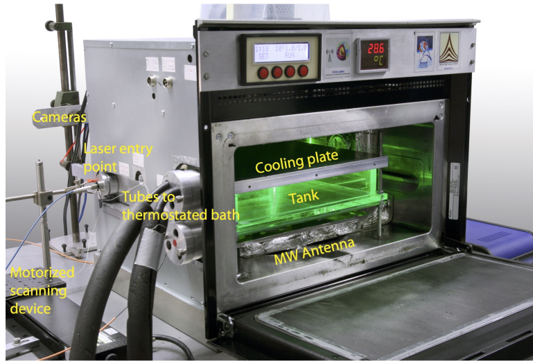
FIGURE 1 – Picture of the setup used in this study (taken from Limare et al. [2019]).
