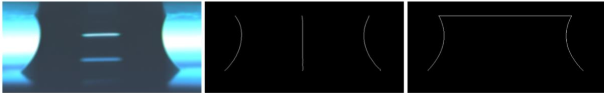
Figure S1: The first image is a single frame directly from the video. The second image is the raw data points for the bridge shape and midline of the bridge. The third image is the fitted polynomials with the receiving contact diameter.
