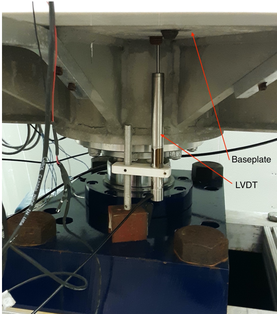
Fig S1. LVDT location. The LVDT is installed vertically and normal to the baseplate that supports the ice chamber (Fig. S3) and moves up or down with it. As the ice chamber moves up and down, the LVDT's spring loaded plunger is pushed out or in. The body of the LVDT is fixed.
