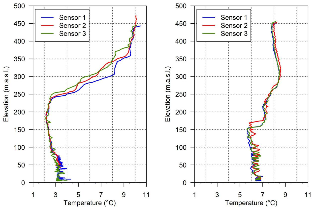
**Fig. S1.** Two ascents five hours apart with all three iMet-XQ2 sensors used in this study. Left: Ascent one, sensor 2 on the UAV, sensors 1 and 3 on a string about 35 meters below the UAV. Right: Ascent two: All three sensors were attached to a string 35 meters below the UAV. Both measurements covered an altitude up to about 450 m a.s.l.
