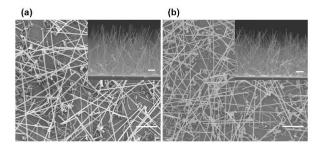
**Figure S1:** SEM images of Ge nanowires grown on the  $SiO_2$  surface, with annealing at 320 °C (a) and 400 °C (b). SEM images were taken with a 25° inclination from the plan-view (in a, b and c) and in cross-sectional view (insets to a, b and c). All scale bars are 1  $\mu$ m.
