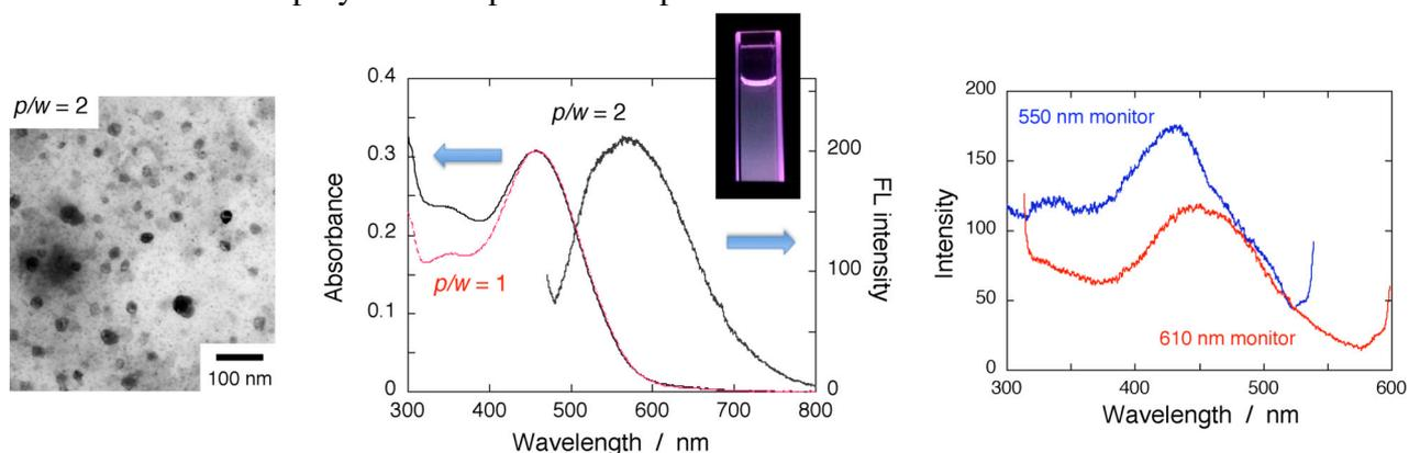
**FIG. S1.** (Left) Typical STEM image, (middle) absorption and fluorescence spectra, and (right) excitation spectra of the MPS-PPV polymer nanoparticles prepared under the condition of  $p/w = 2$  using the NAPA approach.
