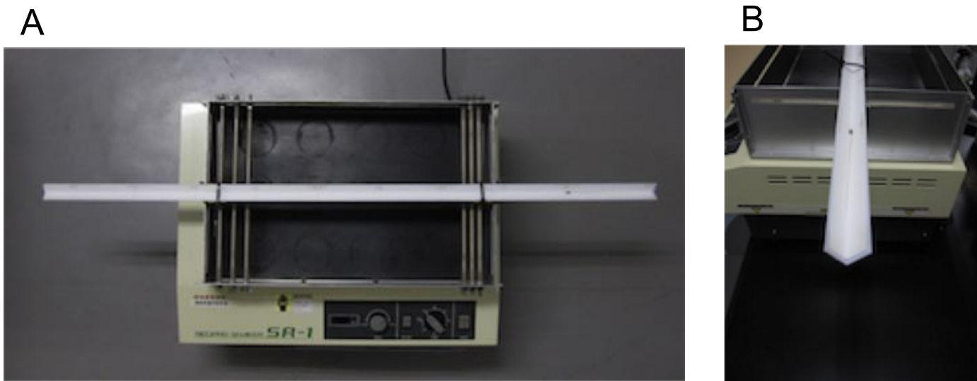
Figure S4. An apparatus for the experiment of horizontal movement on the ground. (A) Top view. A V-shaped plastic rod (80 cm) was set on a reciprocal shaker with a swing of 5 cm. (B) Side view of the rod. The filter paper was fixed on the rod (2 x 2 cm).
