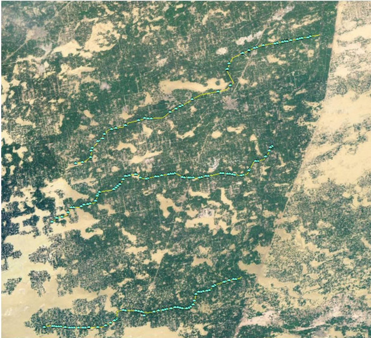
Figure A.1. Overhead view of the Hakra Branch Canal with three secondary channels (in yellow) and outlet locations (light blue dots)
