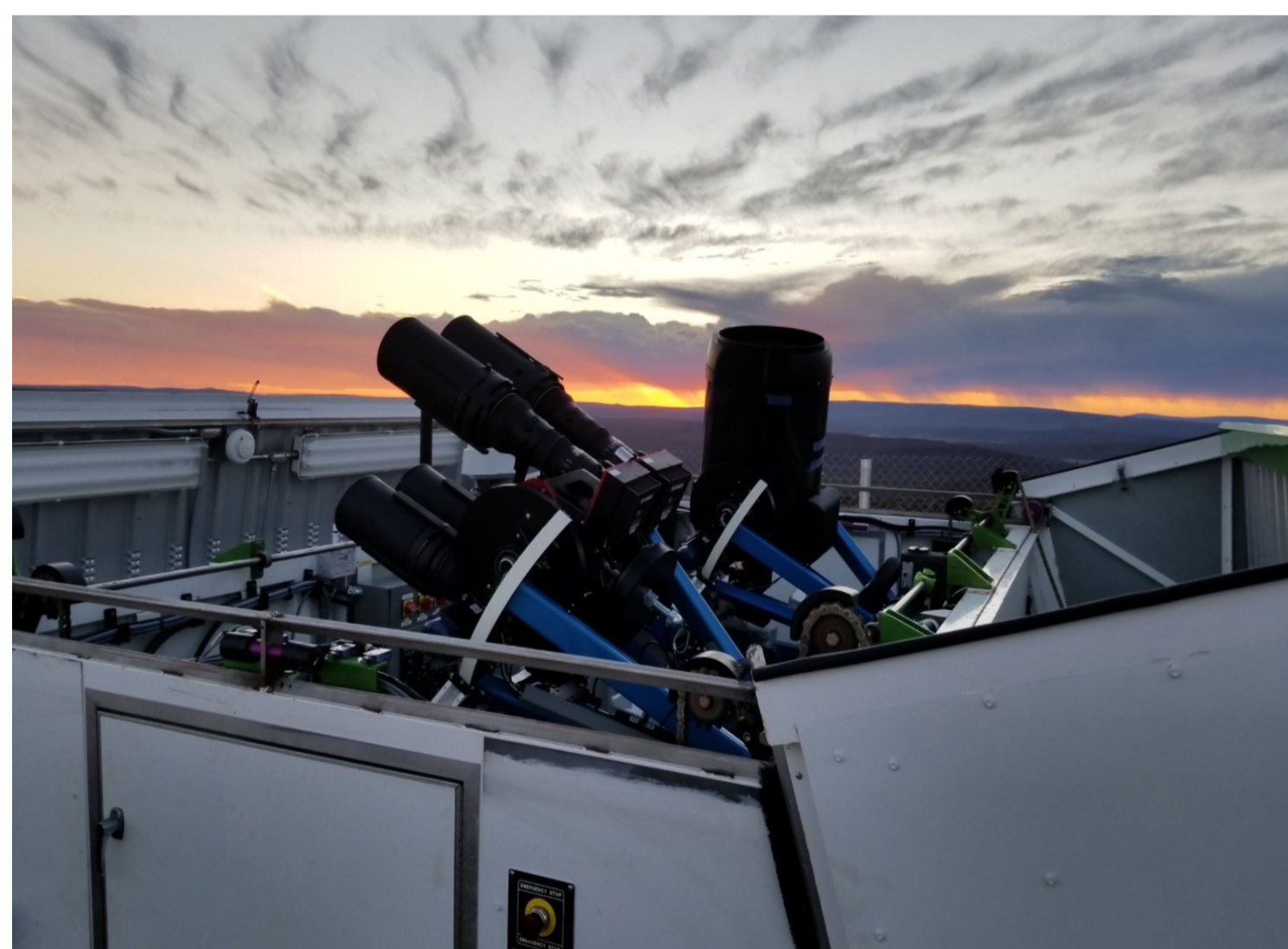
Figure 2: “Payne-Gaposchkin” telescope located at the Las Cumbres Observatory’s South African site. Each unit consists of 4x400 mm Nikon lenses accompanied with 2kx2k Finger Lake CCDs, providing a pixel scale of 7.8” per pixel.
