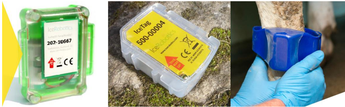
Figure S2. Pictures of the IceTag® sensor (IceRobotics Ltd, Edinburgh, UK) put on the steers to monitor activity. The first picture represents the sensor, the second is the cover to protect the sensor and the third picture shows the exact location on the steers' legs. Copyright: IceRobotics Ltd.
