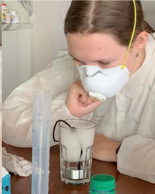
(left) Testing KN95 and N95 masks w/o enclosure (open air) and mist maker.
