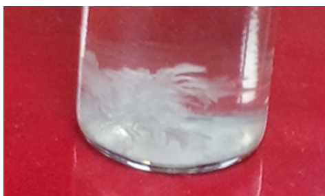
Figure SI-9. Photograph of crystals formed from supernatant S1 after refrigerating at 4°C.
